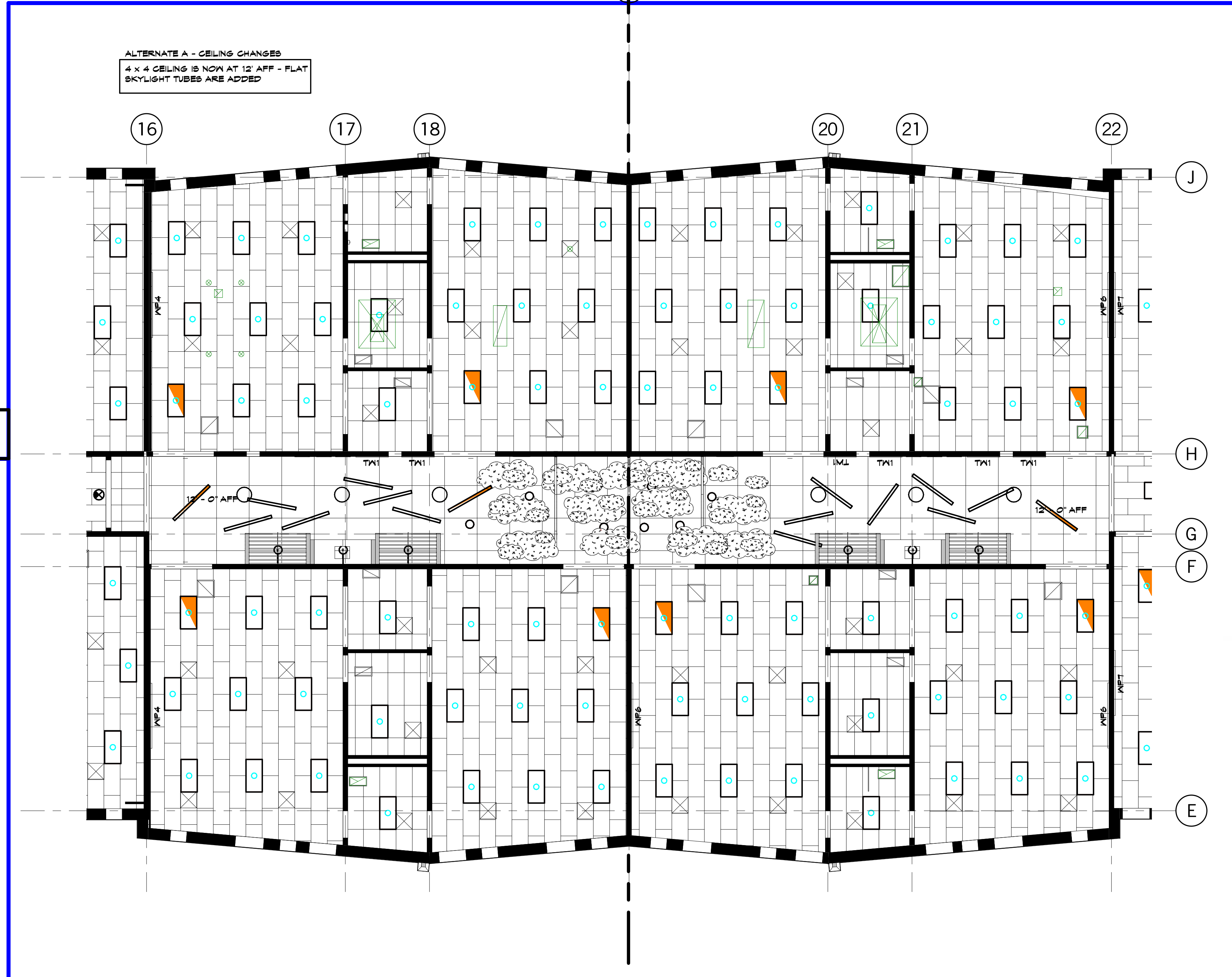
A10 Scale Reflected Ceiling Plan - Alternate A 1/8" = 1'-0"
