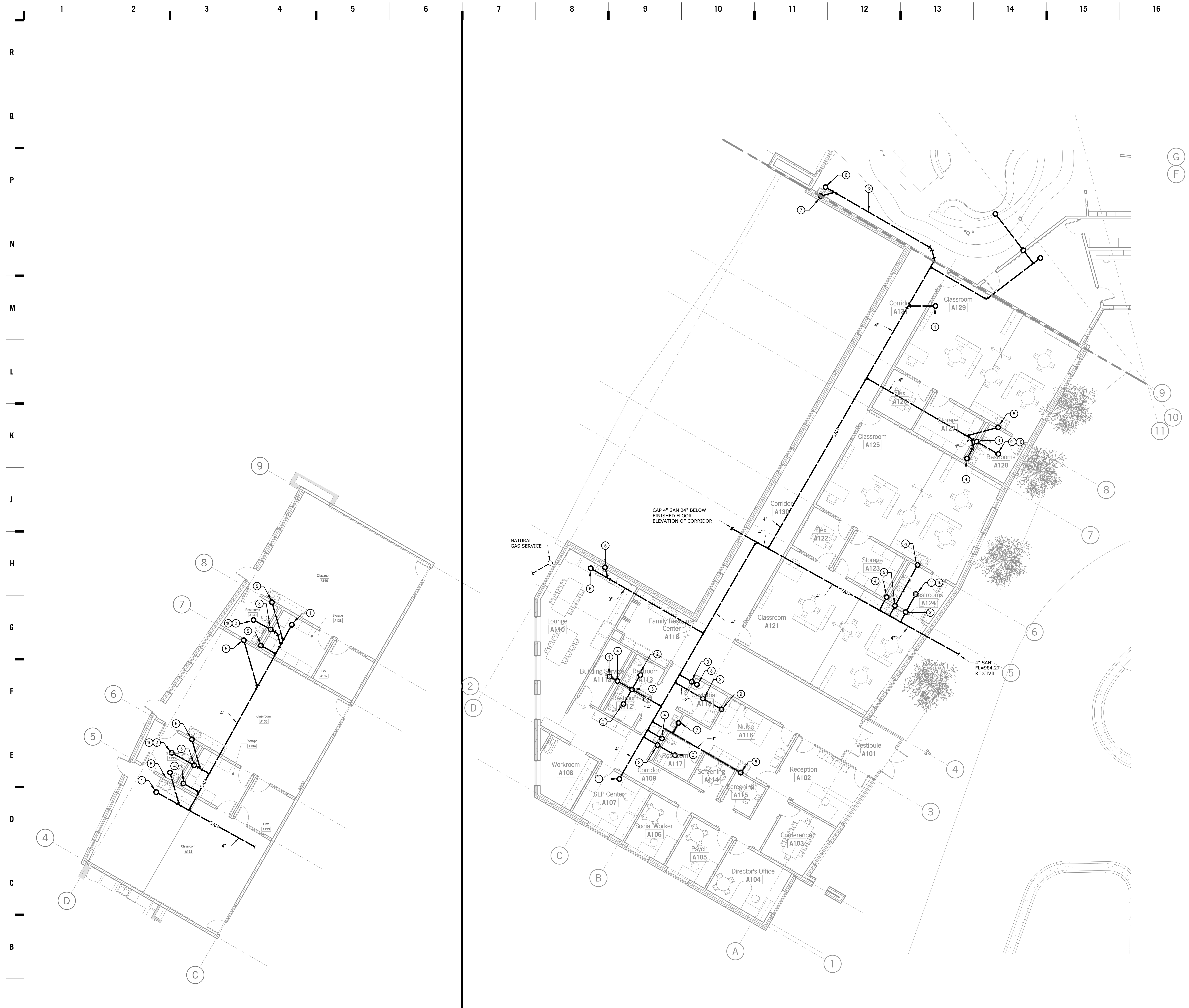
A1 Scale 1/8" = 1'-0" UNDERSLAB FLOOR PLAN - AREA A - ALTERNATE 2 - PLUMBING
