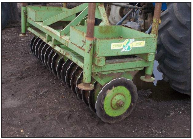
Figure 6.27 Crimping disc. Source: ABCs of BMPs, LLC.
