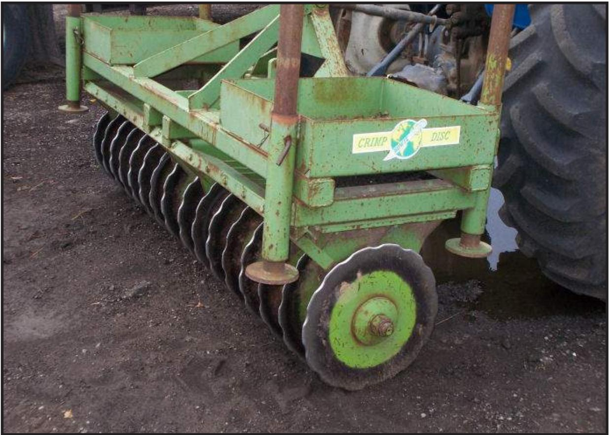
Figure 6.27 Crimping disc. Source: ABCs of BMPs, LLC.
